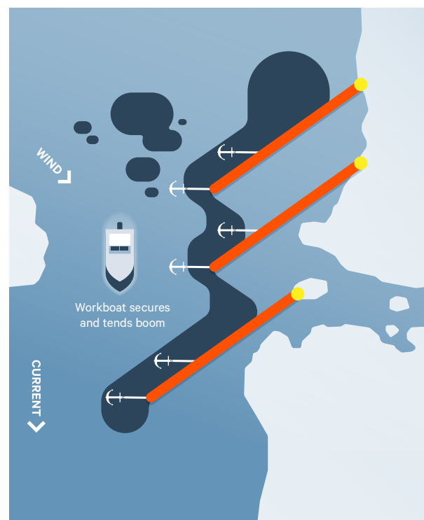
Figure 15: Protective strategy to deflect oil away from the shore.
