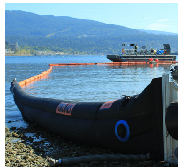
Figure 24: Shore-seal boom being deployed during a training exercise
