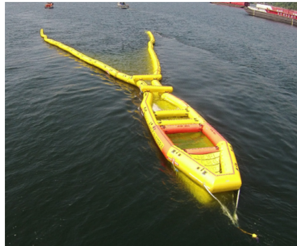
Figure 21: NOFI Current Buster Sweep System
